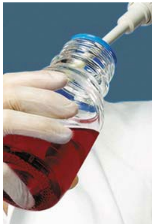
Fig 12. A well-made 40 nm gold colloid shows a typical cherry-red color.
