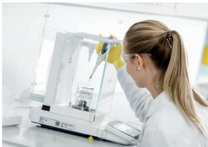
Figure 1: Gravimetric Calibration of a Pipette on a Single Channel Balance
