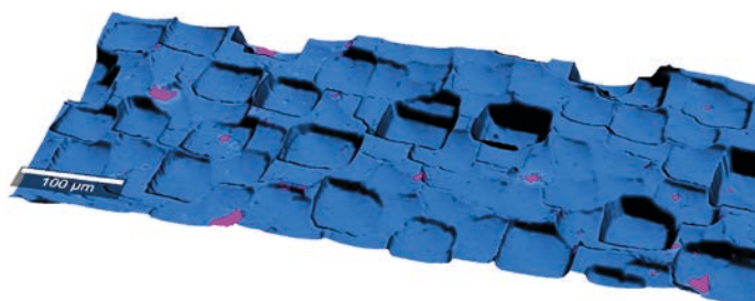
Figure 4: Topographic Raman image of a silicon microstructure.
