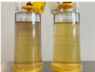
Figure 3: Exemplary results of negative canisters filled with FTM (left) or TSB (right).
